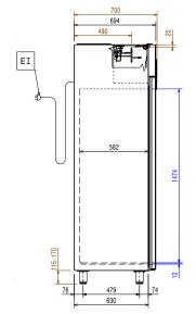
Electrical inlet (power) Refrigerant Inlet RO Refrigerant Outlet
